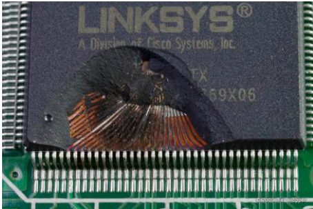
Component damage from a lightning strike
