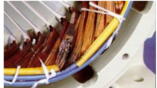
Transient overvoltage impact on motor stator winding
